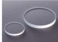
Used as transparent barriers for sending and receiving light between two phases under varying conditions in temperature, pressure, chemical composition, cleanliness, and phase. BK7 windows are used for visible and near IR. AR coated BK7 windows allowed more than 99% transmittance comparing with 92% of uncoated one.
